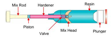
Maximum fluid capacity inside 6" rod = 9cc Maximum fluid capacity inside 8" rod = 12cc
