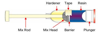
**INJECTION KIT**: For compound with a volumetric ratio of 10 parts or less per 100. The hardener is contained inside the valve mix rod while the resin is in the cartridge.
