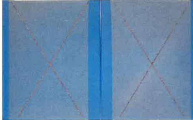
Figure 1 | Scribe Corrosion Test: 2000 Hours Exposure to Salt Spray per ASTM B 117 and ASTM D 1654 on 2024-T3 Aluminum Bare, 0.2 mil (5 µm) primer thickness
